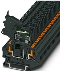
Fuse modular terminal block, fuse type: Glass / ceramics / ..., fuse type: G / 5 x 20, nom. voltage: 250 V, nominal current: 6.3 A, connection method: Push-in connection, 1 level, Rated cross section: 4 mm<sup>2</sup>, cross section: 0.2 mm<sup>2</sup>- 6 mm<sup>2</sup>, mounting type: NS 35/7,5, NS 35/15, color: black
