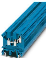
1-level terminal block with double connection on one side, cross section: 0.2 - 2.5 mm<sup>2</sup>, AWG: 30 - 12, width: 5.2 mm, color: blue
