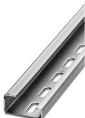
DIN rail perforated, Pack of 10 (20 m), acc. to EN 60715, material: Steel, galvanized, passivated with a thick layer, G profile, color: silver
