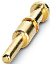
Crimp contact, Pin, turned, contact diameter: 2 mm, crimp range: 0.25 mm<sup>2</sup> ... 1 mm<sup>2</sup>, Alternative product in accordance with RoHS II without Exemption 6c (Pb < 0.1 %) item no.: 1242329
