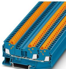
Feed-through terminal block, nom. voltage: 800 V, nominal current: 24 A, number of connections: 3, connection method: Quick connection, 1 level, Rated cross section: 2.5 mm<sup>2</sup>, cross section: 0.5 mm<sup>2</sup> - 2.5 mm<sup>2</sup>, mounting type: NS 35/7,5, NS 35/7,5, color: blue
