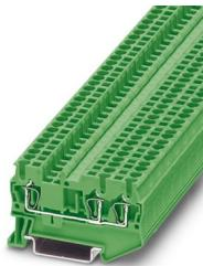
Feed-through terminal block, nom. voltage: 800 V, nominal current: 24 A, number of connections: 3, connection method: Spring-cage connection, Rated cross section: 2.5 mm<sup>2</sup>, cross section: 0.08 mm<sup>2</sup> - 4 mm<sup>2</sup>, mounting type: NS 35/7,5, NS 35/15, color: green
