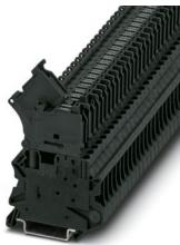
Fuse modular terminal block, fuse type: Glass / ceramics / ..., fuse type: G / 5 x 20, nom. voltage: 250 V, nominal current: 6.3 A, connection method: Screw connection, Rated cross section: 4 mm<sup>2</sup>, cross section: 0.14 mm<sup>2</sup> - 6 mm<sup>2</sup>, mounting type: NS 35/7,5, NS 35/15, color: black
