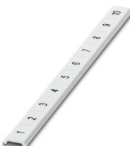
Zack Marker strip, flat, Strip, white, labeled, printed horizontally: consecutive numbers 1 ... 10, 11 ... 20, etc. up to 101 ... 110, mounting type: snapped, for terminal block width: 8 mm, lettering field size: 5.15 x 8.15 mm, Number of individual labels: 10
