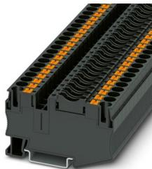
Fuse modular terminal block, fuse type: Flat, fuse type: Type C / max. 2.2 W, nom. voltage: 400 V, nominal current: 25 A, connection method: Push-in connection, Rated cross section: 6 mm<sup>2</sup>, cross section: 0.5 mm<sup>2</sup> - 10 mm<sup>2</sup>, mounting type: NS 35/7,5, NS 35/15, color: black
