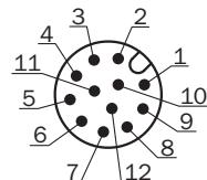
Connecting cable with male connector or M12 male connector, 12-pin, A-coded
