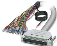
Assembled shielded round cable; connection 1: Single wires (37-position) (The wires are marked and fitted with ferrules. The braided shield is routed to a separate cable end.); connection 2: D-SUB socket strip (1x 37-position); cable length: 1 m
