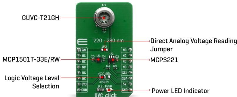
Communication to the MCP3221 is performed using a 2-wire, I2C compatible interface. Standard (100 kHz) and Fast (400 kHz) I2C modes are available with the device. An on-chip conversion clock enables independent timing for the I2C and conversion clocks.
