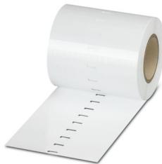
Marker for terminal blocks, Roll, white, unlabeled, can be labeled with: THERMOMARK ROLL 2.0, THERMOMARK ROLL, THERMOMARK ROLL X1, THERMOMARK ROLLMASTER 300/600, THERMOMARK X1.2, THERMOMARK S1.1, perforated, mounting type: snapped, snap into flat marker groove, for terminal block width: 6.2 mm, lettering field size: 6.35 x 6.15 mm, Number of individual labels: 16000
