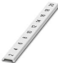
Zack Marker strip, flat, Strip, white, labeled, printed horizontally: consecutive even numbers 2 ... 20, 22 ... 40, etc. up to 82 ... 100, mounting type: snapped, for terminal block width: 6.2 mm, lettering field size: 5.15 x 6.15 mm, Number of individual labels: 10
