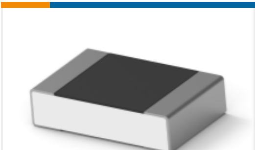
TE Part # 3-2176381-5 RQ 0805 28K 0.1% 10PPM 5K RL
