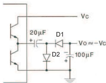
Figure 4. Charge Pump Circuit
