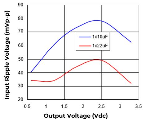
**Figure 40. Input ripple voltage for various output voltages with  $1 \times 10 \mu F$  or  $1 \times 22 \mu F$  ceramic capacitors at the input (2A load). Input voltage is 5V.**
