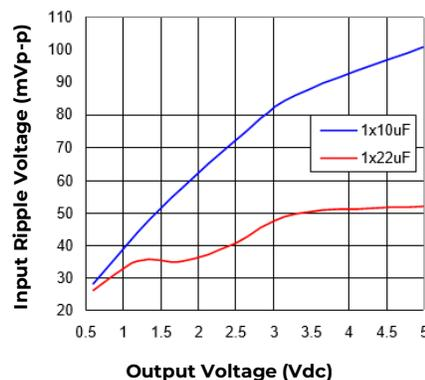
**Figure 41. Input ripple voltage for various output voltages with  $1 \times 10 \mu F$  or  $1 \times 22 \mu F$  ceramic capacitors at the input (2A load). Input voltage is 12V.**
