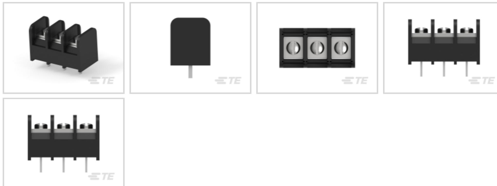
Barrier Strip Style: **Dual Barrier**Bottom Termination Type: **Printed Circuit Pin**Connector System: **Wire-to-Board**Number of Positions: **3**Centerline (Pitch): **9.53 mm [.375 in]**
