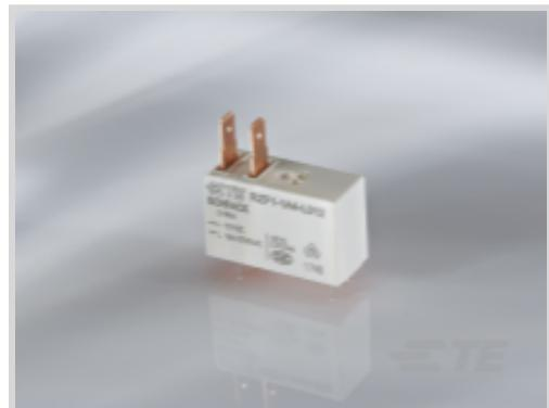
Relay Type: **Standard**Coil Magnetic System: **Monostable**Coil Power Rating DC: **530 mW**Coil Resistance: **4347 Ω**Coil Special Features: **UL Coil Insulation Class F**
