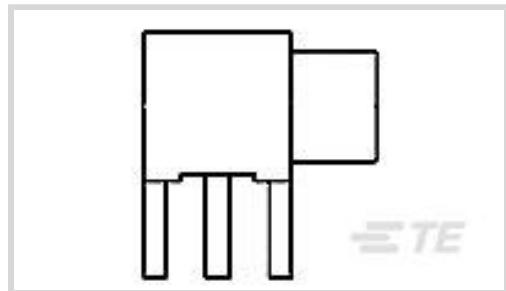
RF Interface: **MCX**RF Connector Style: **Jack**RF Connector Mated Outer Diameter (Approximate): **4.5 mm [.177 in]**Impedance: **50 Ω**RF Connector Coupling Mechanism: **Push-On**
