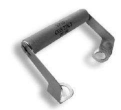
The YP series resistors are coated with multilayer silicone to give an excellent protection to the resistance wire at temperatures from -55°C to 350°C. The terminals are designed for quick and easy mounting on capacitors and have a mounting pitch of 22 and 31.8 mm.
