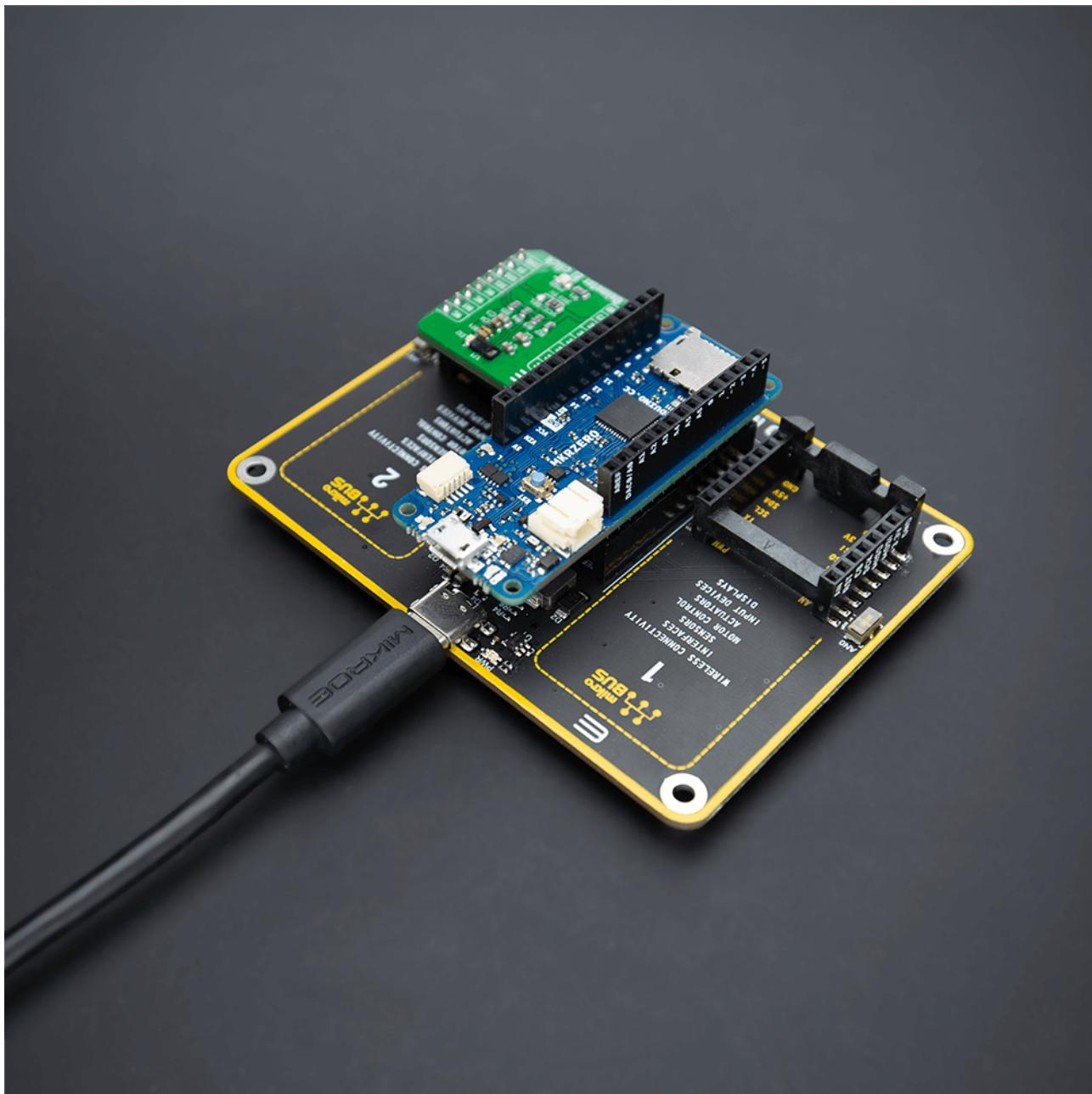
When the USB type C connector is connected to the Shield, the PWR diode will glow Blue, and at this setup, the connected Arduino MKR baseboard and two mikroBUS™ sockets will be powered from it.
