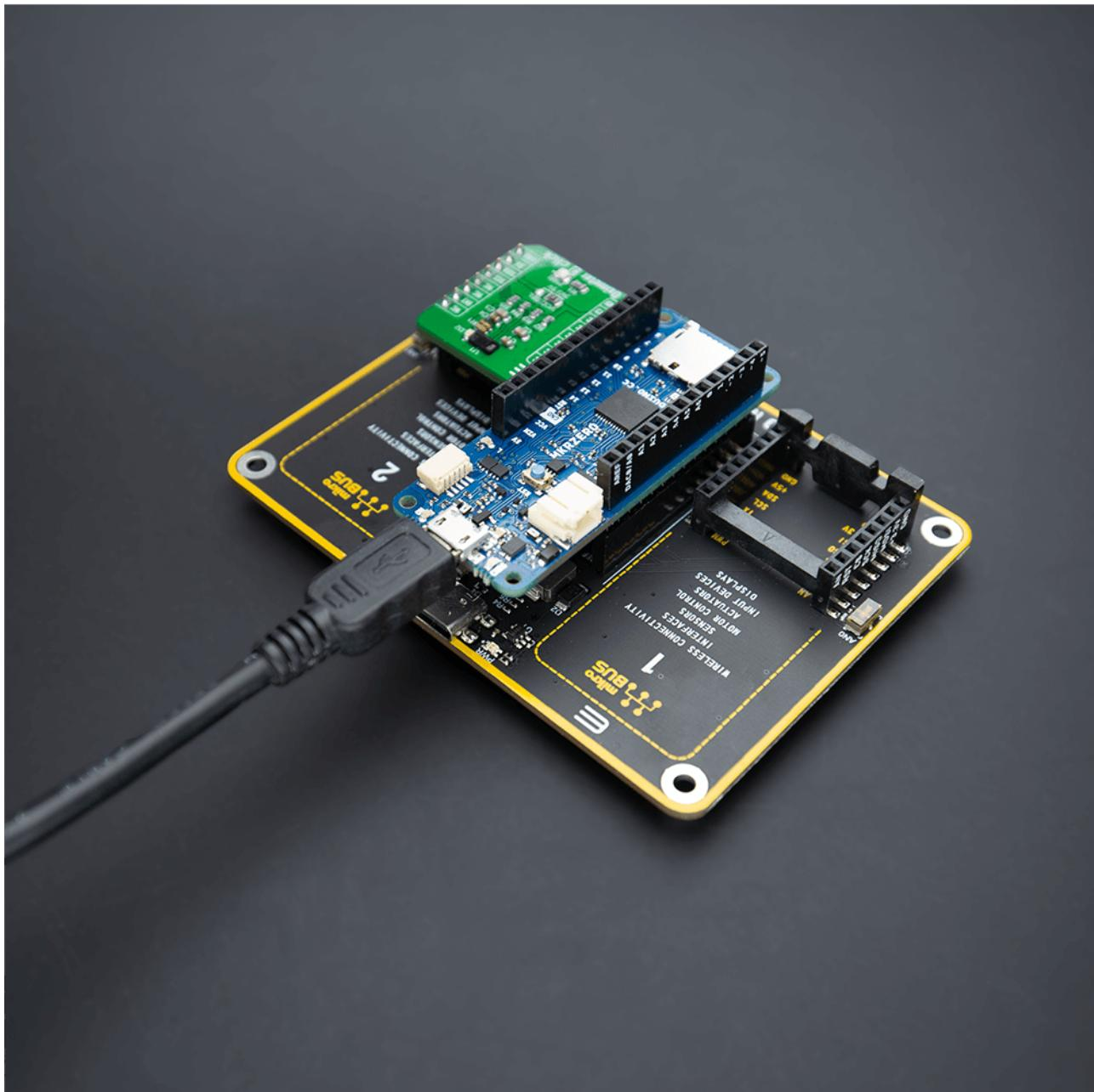
When the USB is connected to the Arduino MKR board, the PWR diode will glow Green, and at this setup, the Arduino MKR baseboard itself will be powered and will provide power to the Shield including two mikroBUS™ sockets.
