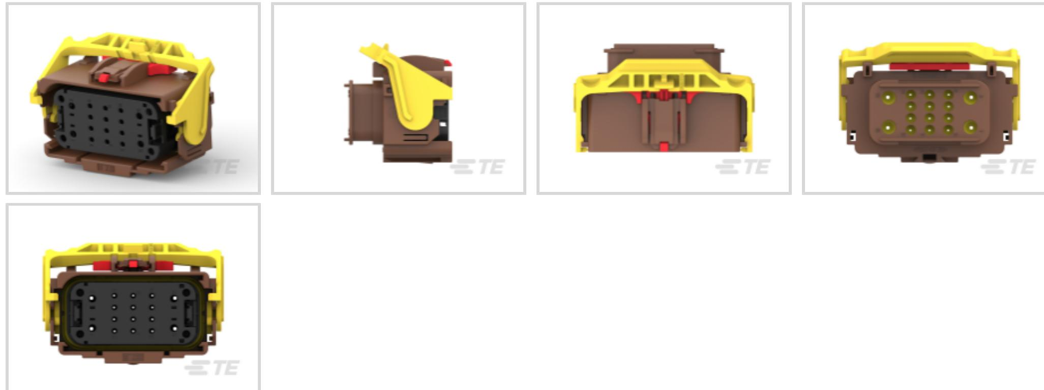
Connector System: **Wire-to-Wire**Number of Positions: **16**Connector & Housing Type: **Housing for Female Terminals**Centerline (Pitch): **7.5 mm**Sealable: **Yes**
