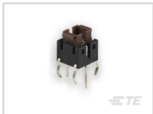
Actuator Style: **Rectangular**Operating Function: **Off (On)**Contact Base Material: **Brass**Switch Contact Plating Material: **Silver**Contact Current Rating: **50 mA**
