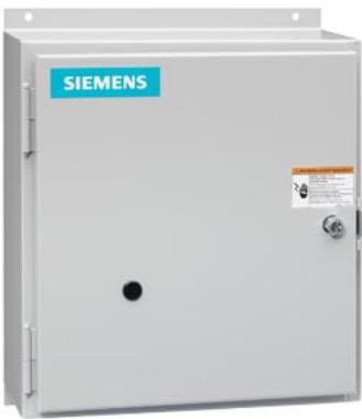
Electrically held lighting contactor, (convertible to mech. held), Amp rating 30A (tungsten 20A), 4 N.C. / 3 N.O. poles, 347V 60Hz coil, Non-combination type, Enclosure NEMA type 12, Dust/drip proof for indoors
