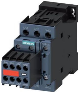
power contactor, AC-3e/AC-3, 32 A, 15 kW / 400 V, 3-pole, 24 V DC, auxiliary contacts: 2 NO + 2 NC, screw terminal, size: S0, captive auxiliary switch, no surge suppressor retrofittable
