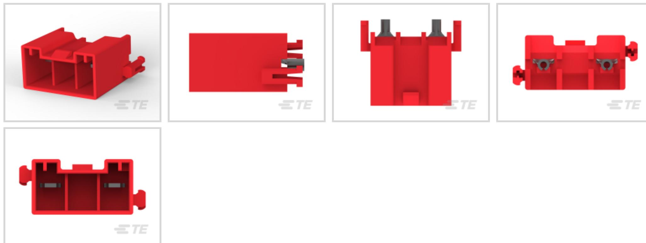
Rectangular Power Connector Type: **Header**Connector & Housing Type: **Receptacle**Connector System: **Wire-to-Board**Number of Positions: **2**Centerline (Pitch): **12.4 mm [.488 in]**
