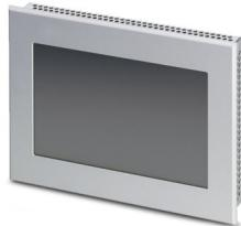
Touch panel with 17.8 cm/7" TFT active display (analog resistive (polyester)), 800 x 480 pixel(s) (WVGA), 262144 colors, Arm® Cortex®-A8, 800 MHz, 2x USB host 2.0, 1 x Ethernet (10/100 Mbps), RJ45, Windows® Embedded Compact 7 and user software: Visu+ / AX OPC Server. (bus system: without)
