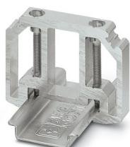
End clamp, for end support of UKH 50 to UKH 240, is pushed onto DIN rail NS 35 and fixed with 2 screws, width: 10 mm, color: aluminum
