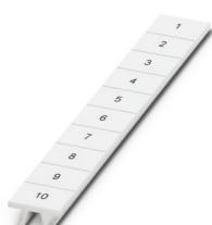
Zack marker strip, Strip, white, labeled, can be labeled with: CMS-P1-PLOTTER, Printed vertically: consecutive numbers 1 ... 10, 11 ... 20, etc. up to 91 ... 100, mounting type: snapped, for terminal block width: 8.2 mm, lettering field size: 10. 5 x 8.15 mm, Number of individual labels: 10
