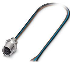
Device connector front mounting, 3-position, Socket, straight, M5, Front mounting, M5 x 0.5, Individual wires, cable length: 0.5 m, 0.14 mm<sup>2</sup>, TPE litz wire
