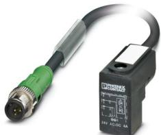
Sensor/actuator cable, 3-position, PUR halogen-free, black-gray RAL 7021, Plug straight M12, coding: A, with 1 LED, on Valve connector CI (9.4 mm), with 1 LED, Wiring: Z diode, cable length: 3 m
