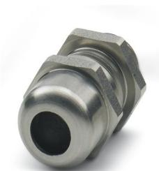
Cable gland, material for screw connection: Stainless steel 1.4305, application: Standard, external cable diameter 6 mm ... 12 mm, shielding: no, connecting thread: M20 x 1.5, color: silver, with O-ring
