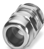
Cable gland, material for screw connection: Brass, nickel-plated, application: Standard, external cable diameter 19 mm ... 28 mm, shielding: no, connecting thread: M40 x 1.5, color: silver, with O-ring
