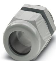
Cable gland, material for screw connection: PA, application: Standard, external cable diameter 19 mm ... 28 mm, shielding: no, connecting thread: M40 x 1.5, color: silver-grey RAL 7001
