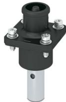
Connector, Range of articles: BPC, color: black, number of positions: 1, min. conductor cross section: 50 mm<sup>2</sup>, max. conductor cross section: 70 mm<sup>2</sup>, rated voltage: 1500, rated current: 250 A, Connection method: Crimp, Contact connection type: Pin
