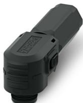
Connector, Range of articles: BPC, color: black, number of positions: 1, min. conductor cross section: 50 mm<sup>2</sup>, max. conductor cross section: 70 mm<sup>2</sup>, rated voltage: 1500, rated current: 250 A, Connection method: Crimp, Contact connection type: Socket, min. cable diameter: 11.3 mm, max. cable diameter: 17 mm
