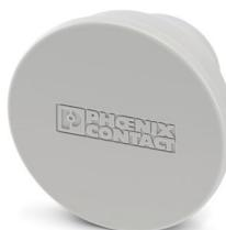
Dust protection cap for energy storage connector, color: gray RAL 7046, ambient temperature for storage and transportation: -40 °C ... 70 °C, operating temperature: -20 °C ... 105 °C, halogen-free, engineering plastics: UL 94 HB, protection class: IP65 (with socket)
