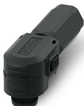
Connector, Range of articles: BPC, color: black, number of positions: 1, min. conductor cross section: 35 mm<sup>2</sup>, max. conductor cross section: 35 mm<sup>2</sup>, rated voltage: 1500, rated current: 160 A, Connection method: Crimp, Contact connection type: Socket, min. cable diameter: 9.7 mm, max. cable diameter: 12.3 mm
