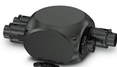
H distributor, Range of articles: PRC 35, design: H-distributor, housing material: Polycarbonate fiber reinforced, color: black, rated voltage: 400 V, rated current: 32 A, Connection method: Preassembled, Contact connection type: Input: pin / outputs: socket, Alternatively, this item can be wired. For your specific requirements, please contact your local PHOENIX CONTACT subsidiary.
