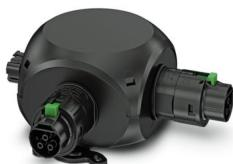
T distributor, Range of articles: PRC 35, design: T distributor, housing material: Polycarbonate fiber reinforced, color: black, rated voltage: 400 V, rated current: 32 A, Connection method: Preassembled, Contact connection type: Input: pin / outputs: socket, Alternatively, this item can be wired. For your specific requirements, please contact your local PHOENIX CONTACT subsidiary.
