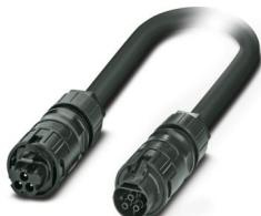
Connecting cable, Range of articles: PRC 35, housing material: PPE, color: black, number of positions: 3, rated voltage: 690 V AC, rated current: 24 A, Connection method: Screw connection, Contact connection type: Socket/pin, This item is also available with other cable lengths. For your specific requirements, please contact your local PHOENIX CONTACT subsidiary.
