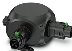
T distributor, Range of articles: PRC 35, design: T distributor, housing material: Polycarbonate fiber reinforced, color: black, max. conductor cross section: 4 mm<sup>2</sup>, rated voltage: 400 V, rated current: 32 A, Connection method: Preassembled, Contact connection type: Input: pin / outputs: socket, Alternatively, this item can be wired. For your specific requirements, please contact your local PHOENIX CONTACT subsidiary.
