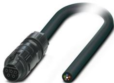
Connecting cable, Range of articles: PRC 35, housing material: PPE, color: black, number of positions: 5, max. conductor cross section: 2.5 mm<sup>2</sup>, rated voltage: 690 V AC, rated current: 32 A, Connection method: Screw connection, Contact connection type: Socket, This item is also available with other cable lengths. For your specific requirements, please contact your local PHOENIX CONTACT subsidiary.
