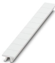
Zack marker strip, Strip, white, unlabeled, can be labeled with: PLOTMARK, CMS-P1-PLOTTER, mounting type: snapped, for terminal block width: 10.2 mm, lettering field size: 10.5 x 10.15 mm, Number of individual labels: 10
