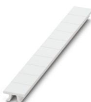
Zack marker strip, can be ordered: Strip, white, labeled according to customer specifications, mounting type: snap into tall marker groove, for terminal block width: 10.2 mm, lettering field size: 10,15 x 10,5 mm, Number of individual labels: 10
