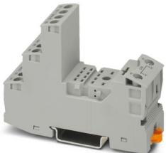
RIF-2.../EX relay base for assembling with RTIII-sealed industrial relays with 4 changeover contacts for use in zone 2, screw connection, plug-in option for input / interference suppression modules, for mounting on NS 35/7,5
