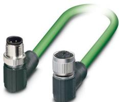
Network cable, PROFINET CAT5 (100 Mbps), EtherCAT® CAT5 (100 Mbps), 4-position, shielded, Plug angled M12 SPEEDCON, coding: D / IP67, on Socket angled M12 SPEEDCON, coding: D / IP67, cable length: Free input (0.2 ... 40.0 m)
