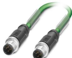
Network cable, PROFINET CAT5 (100 Mbps), EtherCAT® CAT5 (100 Mbps), 4-position, PVC/PVC, green RAL 6018, shielded (Advanced Shielding Technology), Plug straight M12, coding: D / IP67, on Plug straight M12, coding: D / IP67, cable length: 15 m
