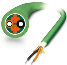
PROFINET polymer fiber cable, duplex, 980/1000 µm, heavy-weight highly flexible design, for flexible cable conduit applications, by the meter, without connector
