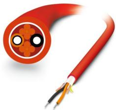
Highly flexible POF round cable (IP20 heads only) for use in drag chains. Individual elements made from extremely wear-resistant polyamide (PA). The cable is halogen-free, ozone and UV resistant, and has a rugged polyurethane (PUR) outer sheath.
