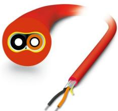
POF installation cable for assembly (IP20 heads only) for installation in stationary systems and machines with individual elements made of polyamide (PA), halogen-free, ozone and UV resistant, with a polyurethane (PUR) outer sheath
