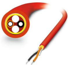
Robust POF installation cable for assembly (IP20 heads only) for installation in stationary systems and machines with individual elements made of polyamide (PA), halogen-free, ozone and UV resistant, with reinforced polyurethane (PUR) outer sheath
