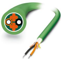
Highly flexible POF PROFINET cable (IP20 heads only) for use in drag chains. Individual elements made from extremely wear-resistant polyamide (PA). The cable is halogen-free, ozone and UV resistant, and has a rugged polyurethane (PUR) outer sheath.
