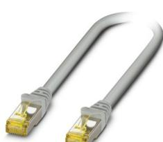
Patch cable, degree of protection: IP20, cable length: 1.5 m, number of positions: 8, 10 Gbps, CAT6<sub>A</sub>, connection method: Pierce connection, connection cross section: AWG 26- 26, cable outlet: straight, Ethernet
