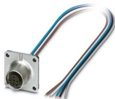
Device connector front mounting, 5-position, Socket, straight, M12, coding: A, on free cable end, Front mounting, Square flange, Individual wires, cable length: 0.5 m, 0.34 mm<sup>2</sup>, TPE litz wire, Alternative product in accordance with RoHS II without Exemption 6c (Pb < 0.1 %) item no.: 1239717
