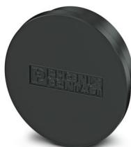
Dust protection cap for energy storage connector , color: black RAL9005, ambient temperature for storage and transportation: -40°C ~70°C, operating temperature: -20°C ~105°C, halogen-free, engineering plastics: UL94 HB, protection class: IP65 (with socket)
