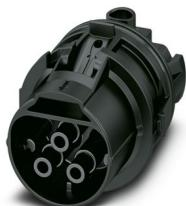
Contact carrier, Range of articles: PRC 35, design: Release with tool or by hand (see accessories), housing material: PPE, color: black, number of positions: 3, min. conductor cross section: 1.5 mm<sup>2</sup>, max. conductor cross section: 6 mm<sup>2</sup>, rated voltage: 690 V AC, rated current: 35 A, Connection method: Screw connection, Contact connection type: Socket, Contact insert without connector housing. Please order the appropriate connector housings according to the accessories list.
