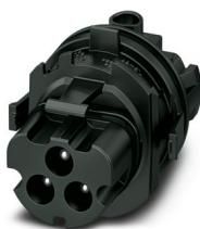
Contact carrier, Range of articles: PRC 35, housing material: PPE, color: black, number of positions: 3, min. conductor cross section: 1.5 mm<sup>2</sup>, max. conductor cross section: 6 mm<sup>2</sup>, rated voltage: 690 V AC, rated current: 35 A, Connection method: Screw connection, Contact connection type: Pin, Contact insert without connector housing. Please order the appropriate connector housings according to the accessories list.
