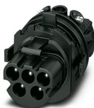
Contact carrier, Range of articles: PRC 35, housing material: PPE, color: black, number of positions: 5, min. conductor cross section: 1.5 mm<sup>2</sup>, max. conductor cross section: 6 mm<sup>2</sup>, rated voltage: 690 V AC, rated current: 35 A, Connection method: Screw connection, Contact connection type: Pin, Contact insert without connector housing. Please order the appropriate connector housings according to the accessories list.
