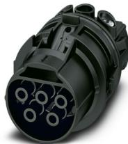
Contact carrier, Range of articles: PRC 35, design: Release with tool or by hand (see accessories), housing material: PPE, color: black, number of positions: 5, min. conductor cross section: 1.5 mm<sup>2</sup>, max. conductor cross section: 6 mm<sup>2</sup>, rated voltage: 690 V AC, rated current: 35 A, Connection method: Screw connection, Contact connection type: Socket, Contact insert without connector housing. Please order the appropriate connector housings according to the accessories list.
