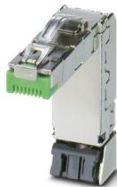
RJ45 connector, design: RJ45, degree of protection: IP20, number of positions: 8, 1 Gbps, CAT5, material: Metal, connection method: Insulation displacement connection, connection cross section: AWG 26- 24, cable outlet: angled, Ethernet
