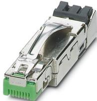
RJ45 connector, design: RJ45, degree of protection: IP20, number of positions: 8, 1 Gbps, CAT5, material: Metal, connection method: Insulation displacement connection, connection cross section: AWG 26- 24, cable outlet: straight, color: green, Ethernet
