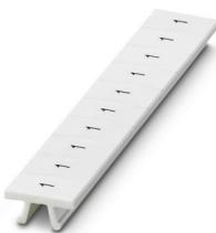
Zack marker strip, Strip, white, labeled, can be labeled with: CMS-P1-PLOTTER, printed horizontally: Identical numbers 1 or 2, etc. up to 100, mounting type: snapped, for terminal block width: 6.2 mm, lettering field size: 6.15 x 10.5 mm, Number of individual labels: 10
