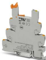
6.2 mm PLC basic terminal block with Push-in connection, without relay or solid-state relay, for mounting on DIN rail NS 35/7,5, 1 changeover contact, input voltage 5 V DC
