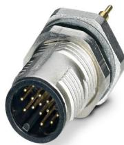
Device connector rear mounting, 17-position, Pin, straight, M12-SPEEDCON, coding: A, Rear mounting, M12 x 1, Solder pins, Alternative product in accordance with RoHS II without Exemption 6c (Pb < 0.1 %) item no.: 1239646
