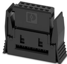
IDC female connector, nominal current: 1.2 A, Test voltage: 500 V AC, number of positions: 68, pitch: 1.27 mm, number of rows: 2, color: black, contact surface: Gold, contact connection type: Socket, For preassembled samples, see the "Accessories" tab.
