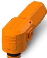
Connector, Range of articles: BPC, color: orange, number of positions: 1, min. conductor cross section: 35 mm<sup>2</sup>, max. conductor cross section: 35 mm<sup>2</sup>, rated voltage: 1500, rated current: 160 A, Connection method: Crimp, Contact connection type: Socket, min. cable diameter: 9.7 mm, max. cable diameter: 12.3 mm
