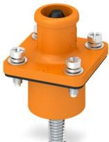
Connector, Range of articles: BPC, color: orange, number of positions: 1, min. conductor cross section: 35 mm<sup>2</sup>, max. conductor cross section: 70 mm<sup>2</sup>, rated voltage: 1500, rated current: 250 A, Connection method: Screw/Solder connection, Contact connection type: Pin
