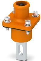
Connector, Range of articles: BPC, color: orange, number of positions: 1, min. conductor cross section: 35 mm<sup>2</sup>, max. conductor cross section: 70 mm<sup>2</sup>, rated voltage: 1500, rated current: 250 A, Connection method: Screw/Solder connection, Contact connection type: Pin
