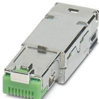
RJ45 male insert, design: RJ45, degree of protection: IP20, number of positions: 8, 1 Gbps, CAT5 (IEC 11801:2002), material: Metal, connection method: Insulation displacement connection, connection cross section: AWG 26- 24, cable outlet: straight, Ethernet
