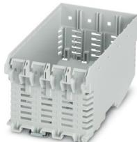
DIN rail housing, Lower housing part with metal foot catch, with vents, width: 75.87 mm, height: 120.6 mm, depth: 64.3 mm, color: light grey (similar RAL 7035), cross connection: DIN rail connector (optional), number of positions cross connector: 5 or 8
