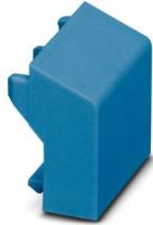
DIN rail housing, Filler plug for unoccupied terminal points (MSTBO), width: 20 mm, height: 19.05 mm, depth: 12.3 mm, color: gentian blue (similar RAL 5010)
