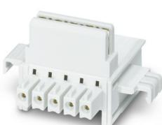
DIN rail connector, color: light grey, nominal current: 8 A (parallel contacts), rated voltage (III/2): 125 V, contact surface: Gold, number of positions: 5, product range: TBUS5-18,8.., pitch: 3.81 mm, mounting: DIN rail mounting, locking: without, mounting: without, type of packaging: packed in cardboard, Item with gold-plated contacts, bus connectors for connecting with electronics housings, 5 parallel contacts
